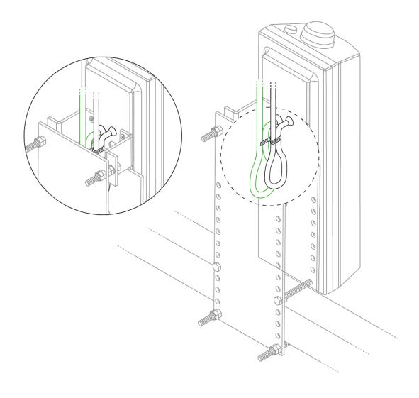
Important: This step ensures that any water droplets are directed away from the cable-case junction. It must not be omitted.
