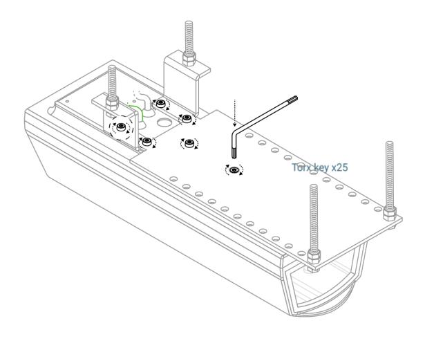
Important: Firmly tighten the screws with the Torx key.
