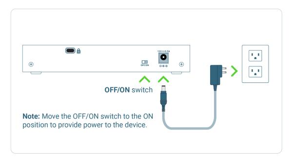
After powering on all connected devices, i.e., the Crane Cameras (and the 4G router if present), monitor the status of the switch. In case of no activity, contact the Crane Camera Support Team at <a href="mailto:construction.support@pix4d.com">construction.support@pix4d.com</a>.
