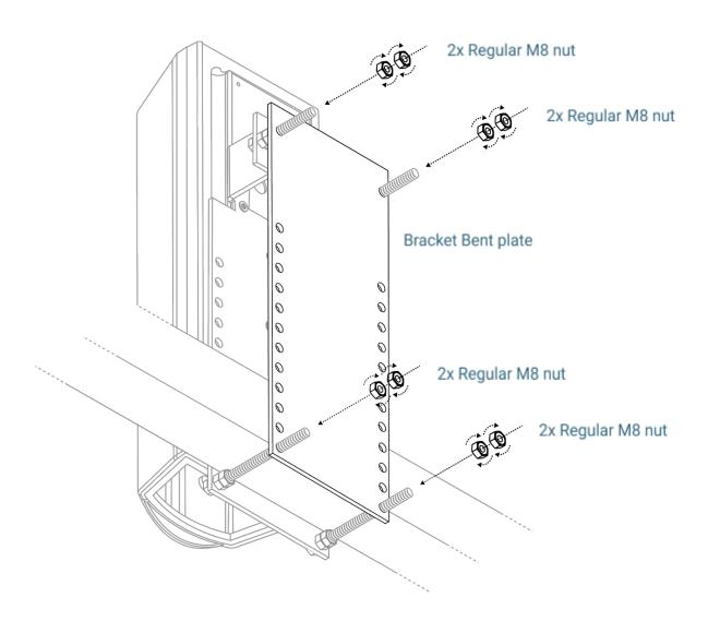
Important: Firmly tighten the M8 nuts.
